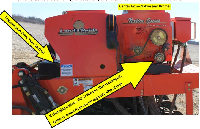
Photo shown with safety cover off. Replace as soon as gears change has been made.
