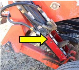
• Once in field, lock in the drive mechanism in the right hand tire hub.
